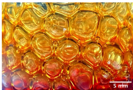
Figure 1: Elastomeric gelatin foam obtained by liquid foam templating
