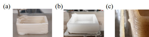
Figure 1: 3D printed objects : (a) Emulsion stabilized by potato proteins (b) Wheat starch suspension (c) Wheat starch suspension including brewer's spent grains
